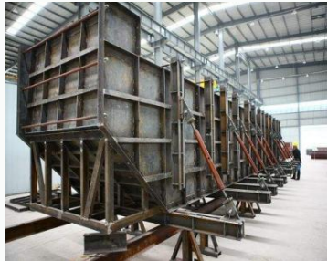
Overpass bent cap formwork
