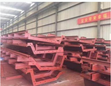
Overpass tie beam formwork
