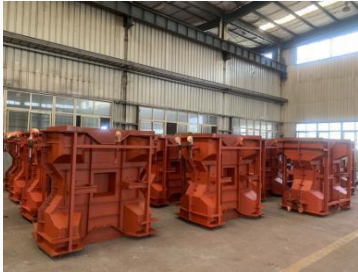
Four corner hollow block formwork
